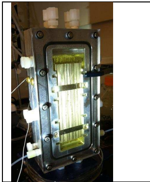
Figure 7 DM's lab-scale electrolyzer
